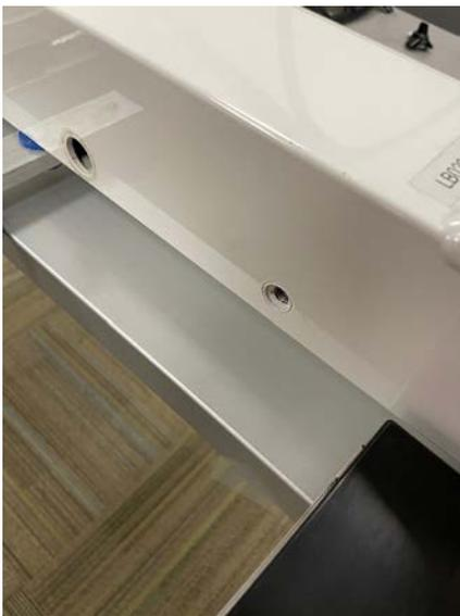
A. Locate the laser post hole on the side of the sewing head and remove the bolt and nut.
