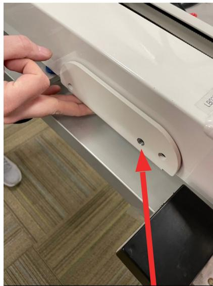
B. Slide the Lower Frame Belt Bracket in between the sewing head and carriage as shown above. Line up the second hole from the right with the laser post hole.
