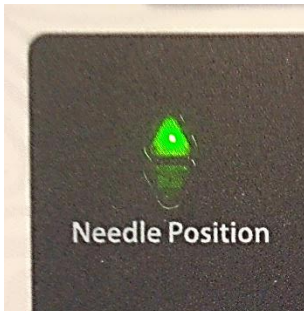
Photo A: Needle will stop “UP”
