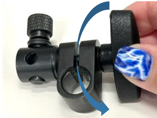
Loosen knob two full turns
