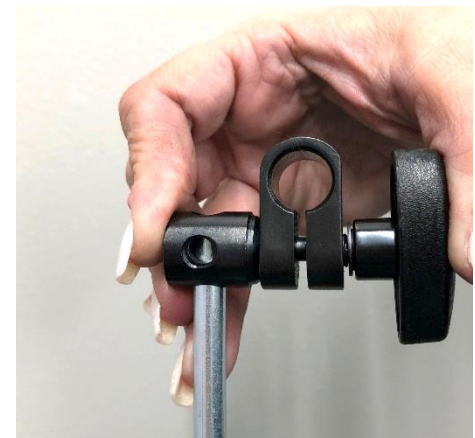
Push clamp onto end of laser post
