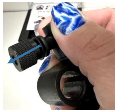
Pull out pin from clamp end
