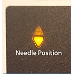
Photo B: Needle will stop “DOWN”
